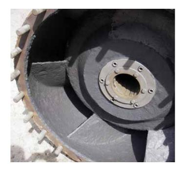
Belzona 1311 (Ceramic R-Metal) is a repair composite designed for rebuilding and protecting metal against the effects of erosion and corrosion.
