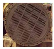
Heat exchanger tube face damaged by severe galvanic and pitting corrosion. Rebuilt with Belzona 1511 prior to the application of a Belzona high temperature coating.
